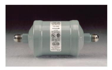
The unique design of the molded desiccant block allows for efficient filtration and retention of solid contaminants, while insuring minimum pressure drop. The molded block exposes maximum surface area and provides even distribution of filtered material as the refrigerant flows through the drier.
